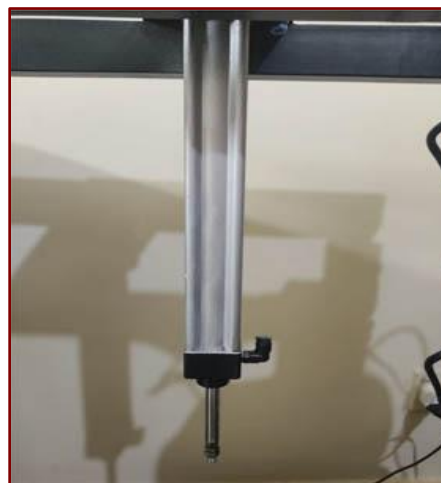
Figure 2: Double Acting Pneumatic Cylinder
