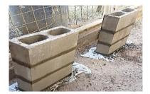
Curing of Masonry Prisms
