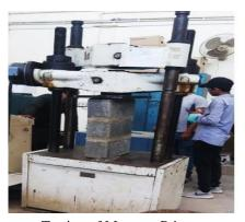
**Testing of Masonry Prisms**
