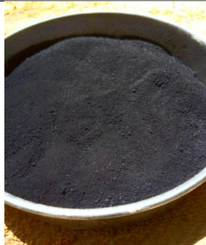
ETP sludge to be used as construction material
