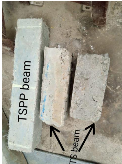
Beam developed using ETP sludge for testing
