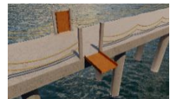
Openable door ramp
