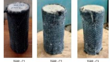
TFRP (T25 Tapanan uni-directional Fabric + Sikadur 30)
